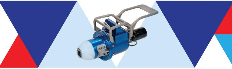
The Class 1-4 Torque Tool is a dependable tool with a reliable Mechanical Counter to avoid the inherent problems associated with electronic digital counters. The robust latch system provides the confidence to be securely locked into the subsea bucket. In the case of an unforeseen power failure, the latches are spring loaded and will
