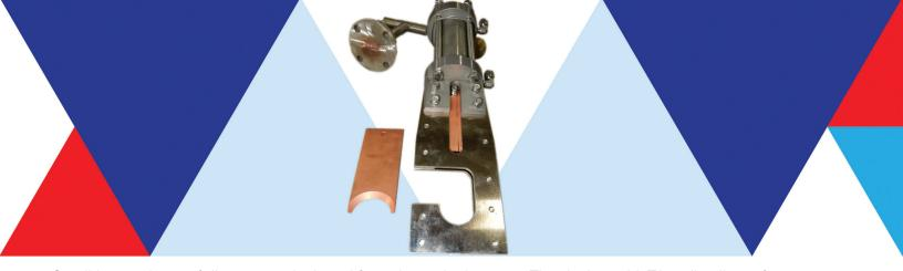
Small heavy duty soft line cutter designed for subsea deployment. The design with T-handle allows for easy deployment by ROV manipulator. Compact design is ideal for operation in confined spaces or where access is limited. The Tool consists of a hardened tool steel blade and side plates, a hydraulic cylinder to actuate the blade. One side of each plates is open to allow the cutter to be placed on the line.
