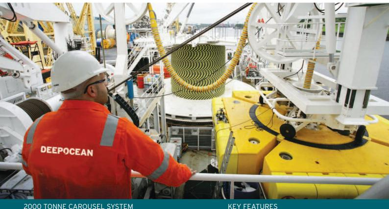
The 2000 tonne rated carousel provides a reliable, efficient and cost effective solution to facilitate the installation and/ or simultaneous burial of flexible products.
