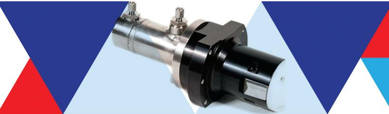
Delta SubSea offers an API/ISO 13628-8 Figure 7 compliant docking probe. The docking probe is hydraulically actuated with an emergency spring return to retract automatically during a dead sub recovery. DSS can also provide the female mating receptacle to be mounted on the tree or pile for orientation purposes.
