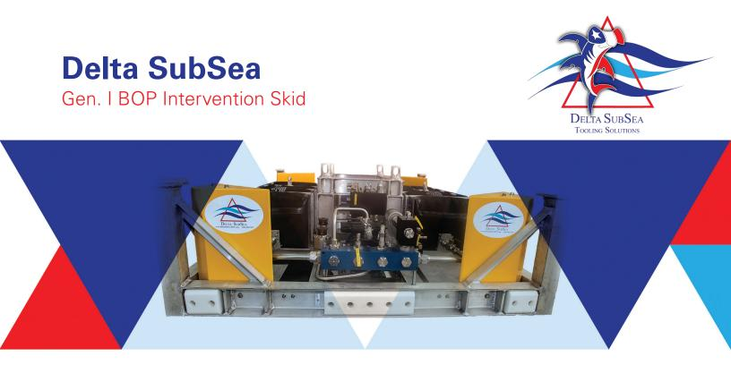
The DSS Gen. I BOP Intervention Skid is an ROV underslung skid mounted BOP intervention device capable of providing BOP fluids at pressures up to 5000 PSI and flows up to 10 GPM. This device is for subsea testing and intervention of BOPs. This design uses software based electronic flow and pressure monitoring.
