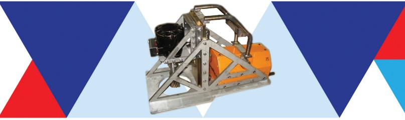
Delta SubSea's hydraulic Mag Drill is designed to accept up to a 6" diameter annular cutter with a 3/4" shank and will easily cut holes into any flat or round steel structure. It will readily allow for a 1", 2" or 3" depth-of-cut annular cutter bit with the maximum travel of the cutter being 4 1/4". The drill is mounted to the work site by energizing a lifting magnet using a hydraulic cylinder as the actuator.
