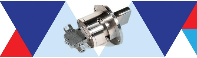
Delta SubSea offers ROV operable ball valve interfaces for the many subsea ball and directional control valves on the market. Construction is all stainless steel, has a 20yr design life and meets the API 17D and 17H specifications for ROV interfaces. The Paddle Valve as its often referred to eliminates the worry of an ROV manipulator damaging the valve stem causing the equipment to be returned to the surface for repair.
