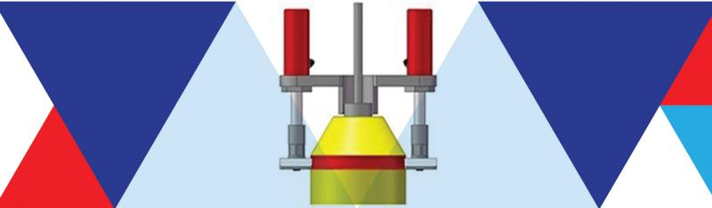
Delta SubSea's GL4 Regan Latch release tool is manipulator deployed and allows an ROV to mechanically attach to the top of the guidepost. It then hydraulically compresses the latching mechanism making it possible to remove the guidepost for retrieval to the surface on the guide wires provided. The GL4 hydraulic supply can be plumbed directly to the ROV or use a hot stab attachment.
