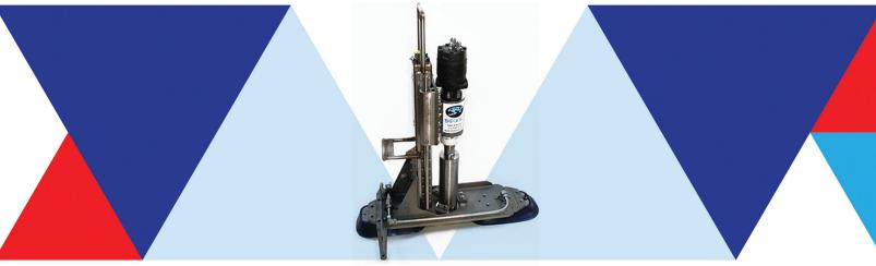
Delta SubSea's hydraulic Core Drill is to make holes in jacket legs and other structures for lifting jig installation, flooding or inspection access. The drill is hydraulically actuated and attaches to the structure via sticky feet suction cups. Capable of being operated by any work class ROV of opportunity.
