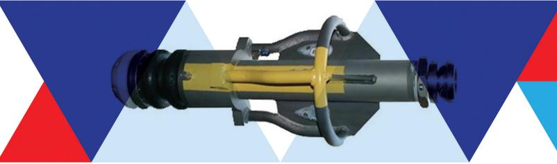
DSS currently offers an ROV friendly Suction Pile Interface Stab. Our robust design has an inflatable seal to overcome the common sealing problems often present in the irregular painted surfaces inside the stab interface of most suction piles. A port has been added, allowing for the easy installation of a differential pressure gauge which can significantly reduce your risk of damaging the suction pile. Each Suction Pile Interface Stab is rigorously tested onshore.
